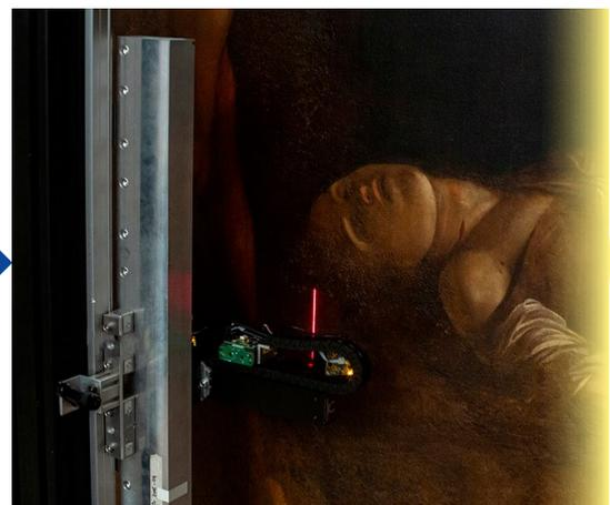
*The Lucida 3D Scanner recording the surface
